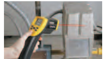
Measuring industrial equipment that is too hot to touch.
